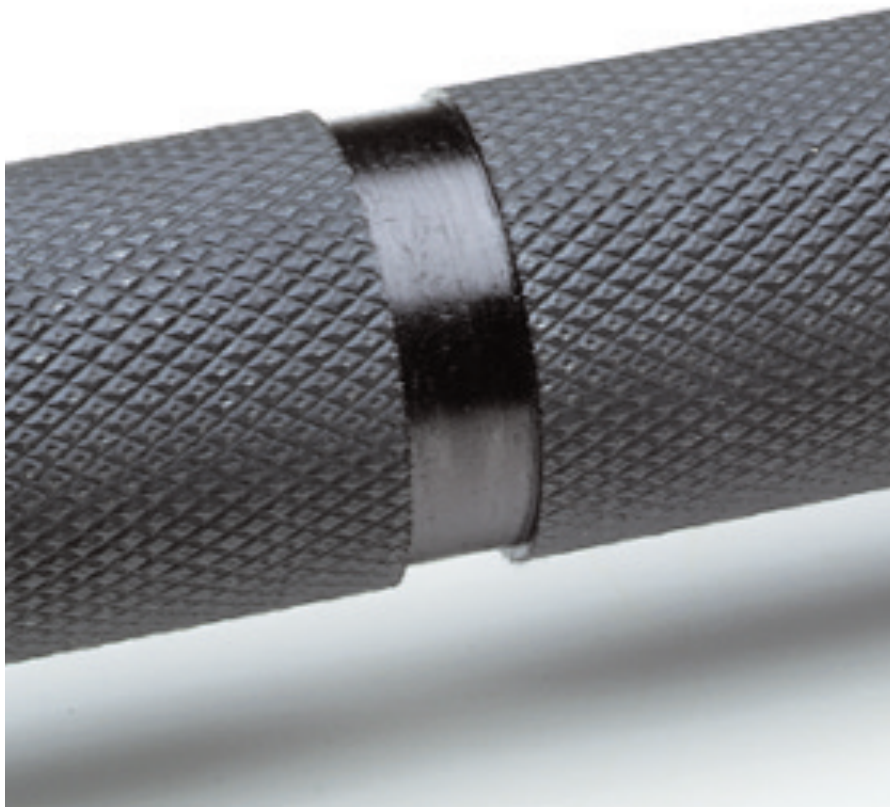
A bar showing a typical “suicide groove”. This cosmetic feature will weaken the bar at this point, and is often the precursor of bar failure.
