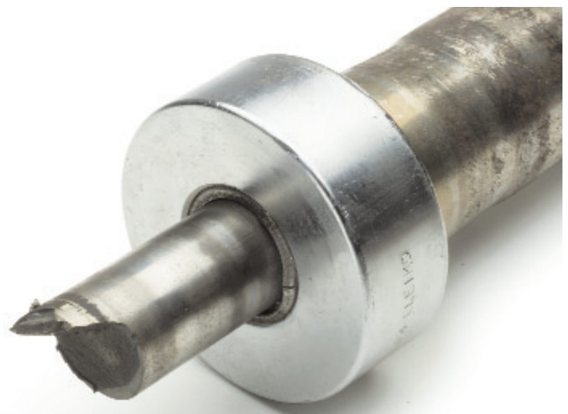
A typical bar failure (snap). Note jagged edge. This is usually the way they break.
